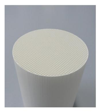
In the drying process, Tylose prevents cracks via its binding effect, additionally supported by its thermal gelation capabilities. For flux sensitive applications, Tylose low sodium grades are recommended.
