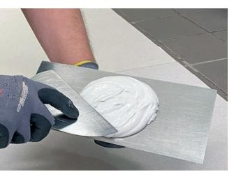
Emulsion based construction products are ready to use paste formulations. These formulations include Tylose® MC (MHEC and MHPC) or Tylose HEC or both. Tylose improves water retention, consistency and adhesion of emulsion based building materials.
