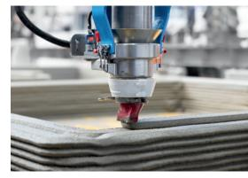
provide the correct rheology: A shear-thinning effect during pumping and good thixotropy (yield point) after processing. In addition, a good wettability between the applied mortar layers is desired to avoid "cold bonds" during hydration.
